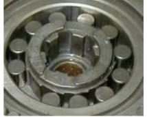
For counterclockwise rotation, the opposite is true. If the annulus is rotating slower than the mainshaft, the rollers go down the ramps and the clutch is released. If the annulus tries to rotate faster than the mainshaft, the rollers go up the ramp and lock the annulus to the mainshaft
