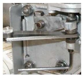
The Haynes manual also specifies an end float on the operating shaft of approximately .008 inch. The end float was checked with the dial indicator and found to be within the approximate .008 inch specification that was interrupted rather broadly.
